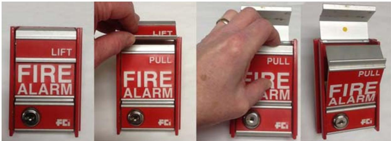
To activate this type of fire alarm pull station, lift up the flap, grasp the top of the device and pull towards you. You will hear a click, and the device will lock into position.
